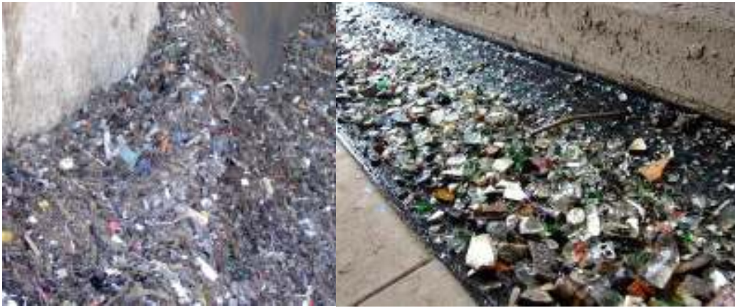
Figure 5 – Contaminants removed by Waste Dissolver (Light and Heavy)
