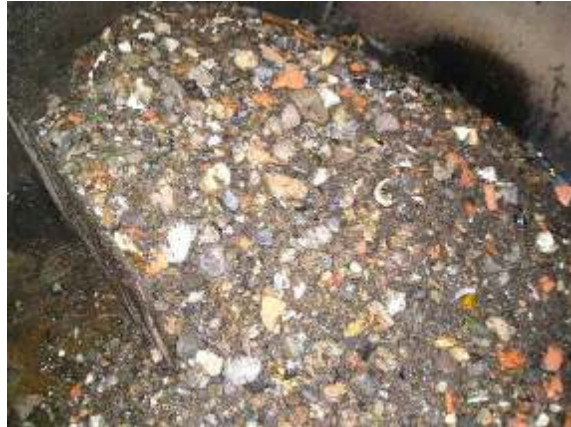
Figure 9 – Heavy Fraction Contaminants from Waste Dissolver
