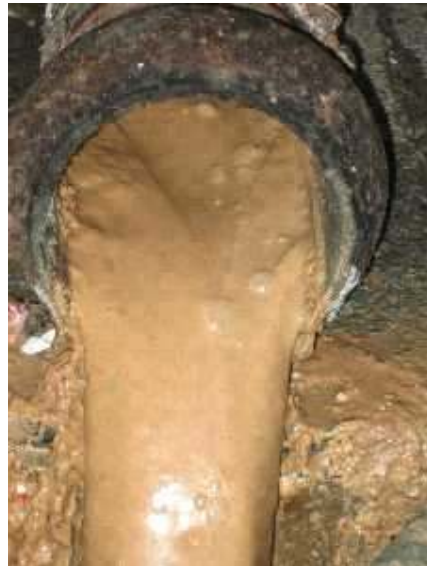
Figure 4 – Organic Slurry from Dissolvers
