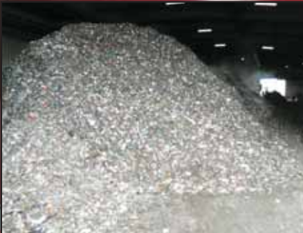
Residual waste feed stockpile - input to dissolvers
